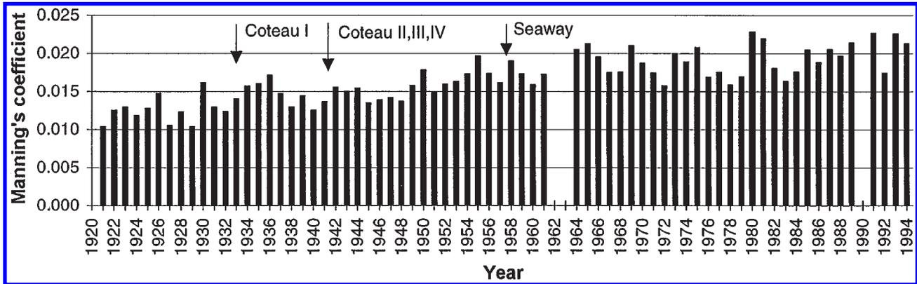
Summerstown is located 35 km upstream from Coteau-Landing on the north side of the river. An aggregated version of Manning's equation was used to estimate the monthly average friction from water level data ( $h(t)$ ):
