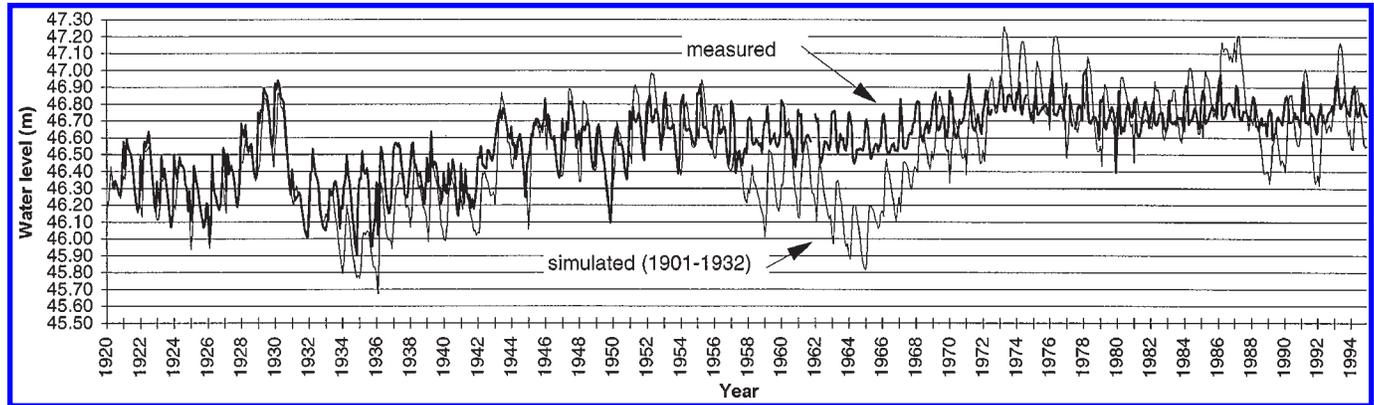
Fig. 16. Natural variations in water level for Lake Saint-François wetlands, simulated from 1901–1932 and from pristine state (pre-1849) stage–discharge relationships.
